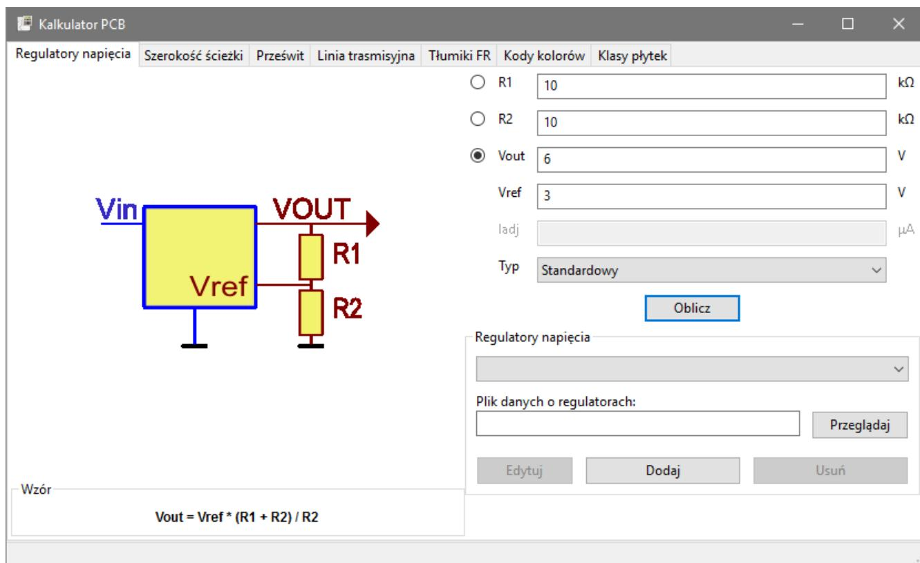
For the *Standard Type*, the output voltage  $V_{out}$  as a function of the reference voltage  $V_{ref}$  and resistors  $R_1$  and  $R_2$  is given by:
